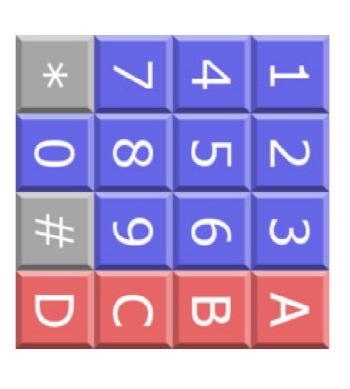
DTMF is used for telecommunication signaling over analog telephone lines.
